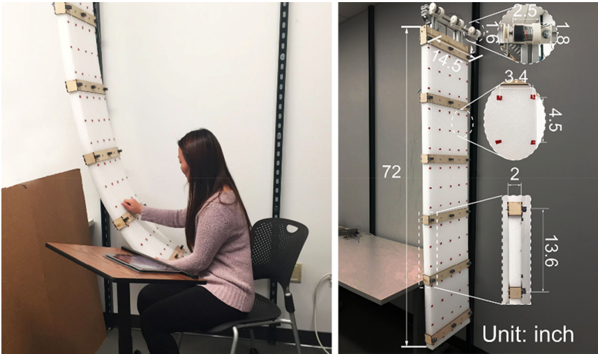
Fig. 1. Our robotic wall (right) prototype and photo from a pilot study with a user (left).
